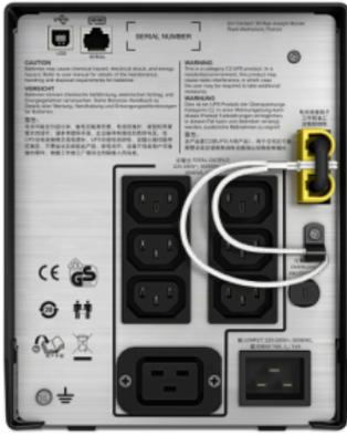
APC Smart-UPS C, Line Interactive, 2000VA, Tower, 230V, 6x IEC C13+1x IEC C19 outlets, USB and Serial communication, AVR, Graphic LCD
